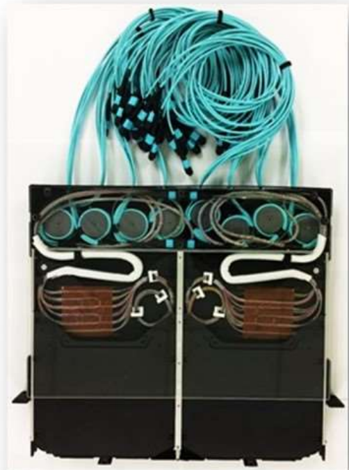
Fiber Flex Circuits in Go!Foton's PEACOC 1RU Fiber Panel
